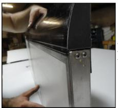
■Step 3: Once the "tab" is located in the channel of the extrusion and the thrower has been rolled over the extrusion, you are ready to secure the vinyl thrower to the wall vent panel.
