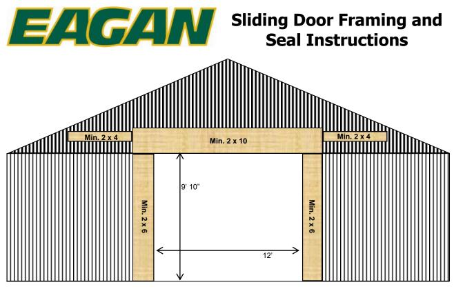
Above is the necessary wood frame work for the Eagan Sliding Door. It requires a minimum 2x6 on each side and a minimum 2x10 header across the top. You may then use 2x4's to extend out from each side of the header for the track installation. Once complete, the remaining rough opening should be exactly 12' x 9'10".
